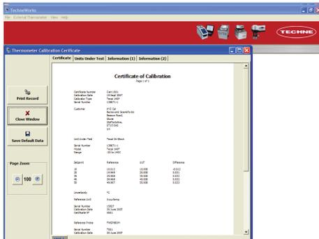
TechneWorks software allows connection to a range of Precision Thermometers such as the Techne Accu-Temp, ASL model F250, Accu-Temp11 and the Cropico 3000 series. TechneWorks software enables you to calibrate thermometers and sensors and to then generate calibration certificates using a Techne Liquid bath or Dry block as a temperature source. The Calibration bath or Dri-Block's display can act as the reference temperature or connect to a range of external thermometers.
